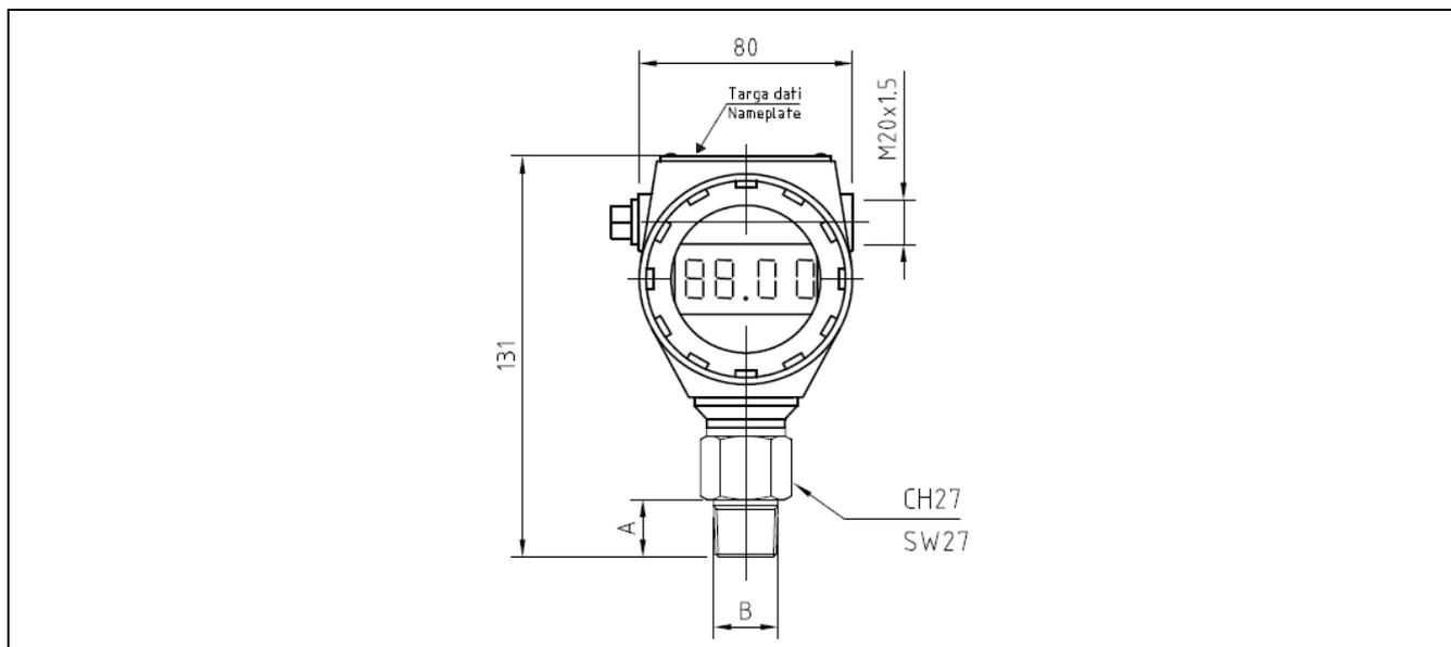
Figure 2 - Attacco filettato / Screwed connection
