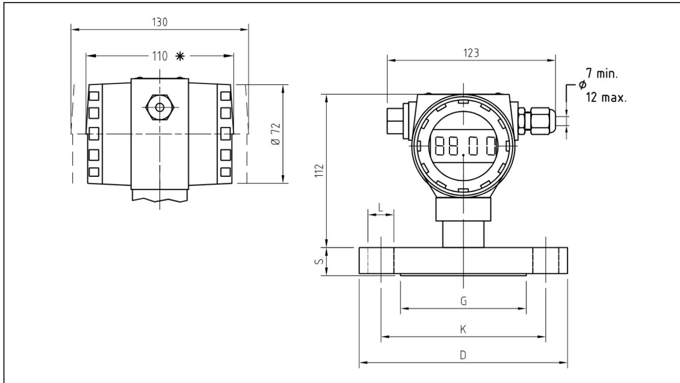
Figure 1 - Attacco flangiato / Flanged connection (UNI, ASME...)
